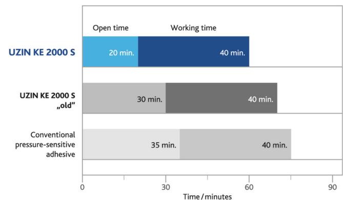
PVC sheet installation on UZIN NC 170 LevelStar, notch size A 2, at 20 °C and 65 % relative humidity.
