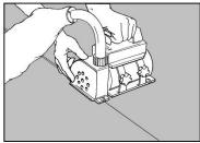
The tiles are hot welded. Do not weld until the adhesive has bonded completely, wait 24-48h. The joints are chamfered or grooved to about 3/4 of the thickness using a hand grooving tool or machine prior to welding.
